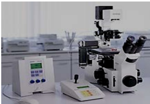
Figure 22. Eppendorf FemtoJet and Micromanipulator on a Nikon TE 2000 Inverted Microscope.
